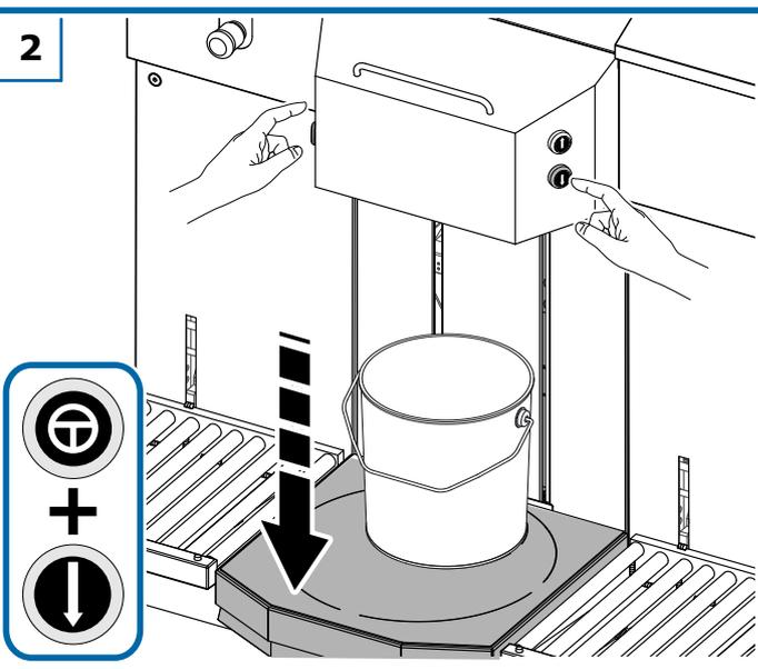
With the purpose to prevent any crushing risks, the semiautomatic shelf is fitted with a lower safety plate (chapter 3.5). The safety plate intervenes by causing the shelf to stop if it is inadvertently touched by the operator.
