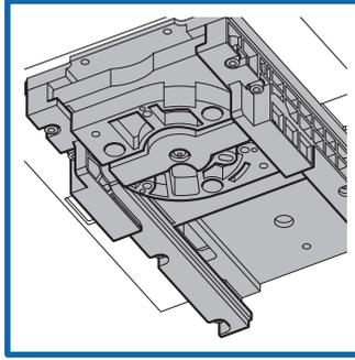
To prevent colorants from drying out in the nozzle center, the machine is equipped with a humidifier cap or a nozzle cleaning device.
