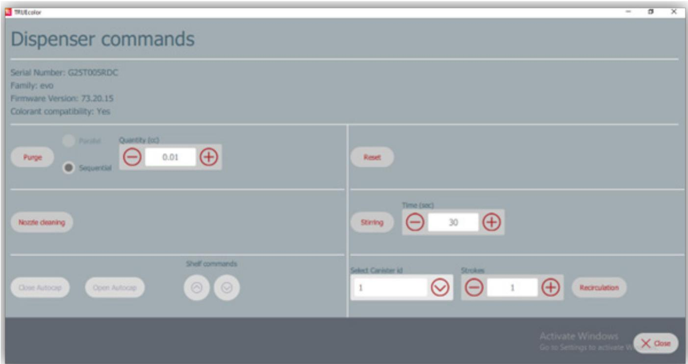
This feature enables T-Series dispensers to recirculate the fluid using a specified number of strokes.
